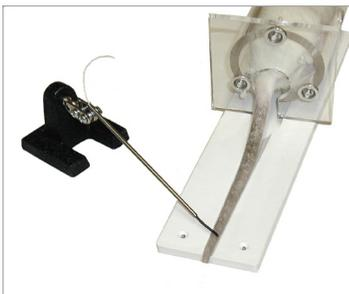
Measurement of tail temperature at all times. Trigger temperature is automatic at start of every test. Warms tail to preset temperature (set by user) and then tests start, allowing all tail temperatures to be identical.
